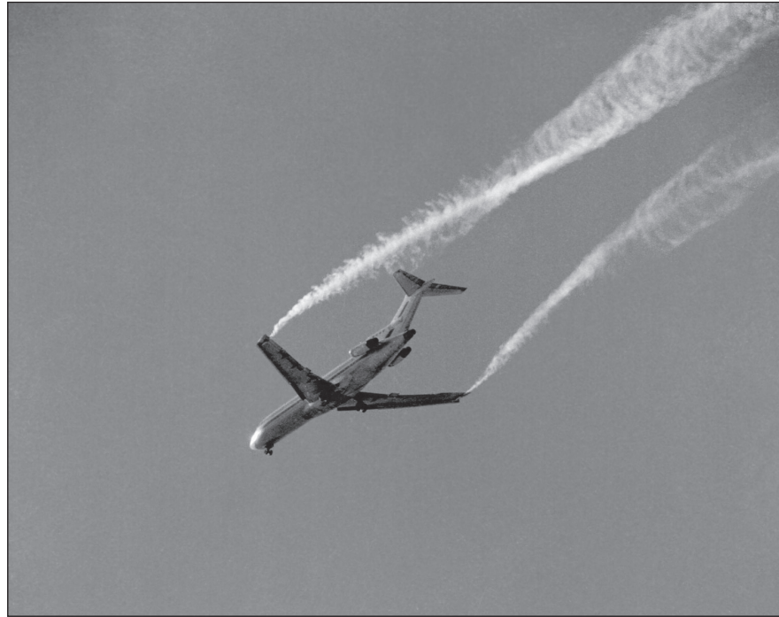
Fig. 8.27 Wingtip vortices from a smoke-visualization test of a Boeing 737. Vortices from large airplanes can be extremely dangerous to any following aircraft, especially small planes. This test was part of a research effort to alleviate these swirling wakes. (NASA)
