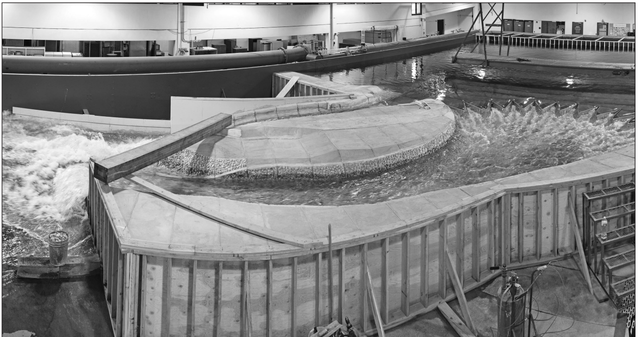
Fig. 5.8 Hydraulic model of the Isabella Lake Dam Safety Modification Project. The model scale is 1:45, and was built in 2014 at Utah State University's Water Research Laboratory. (Courtesy of the U.S. Army photo by John Prettyman/Released.)
