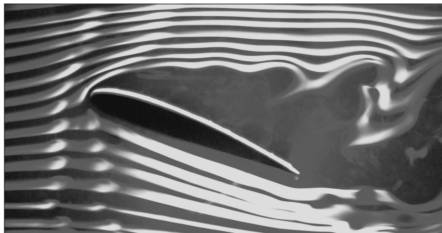
Fig. 7.24 At high angle of attack, smoke flow visualization shows stalled flow on the upper surface of a lifting vane. (Gary S. Settles & Jason Listak/Science Source)
