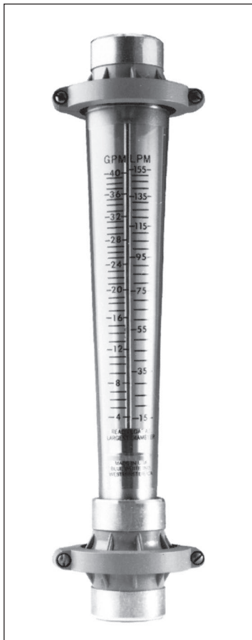
Fig. 6.36 A commercial rotameter. The float rises in the tapered tube to an equilibrium position, which is a measure of the fluid flow rate. (Courtesy of Blue White Industries.)
