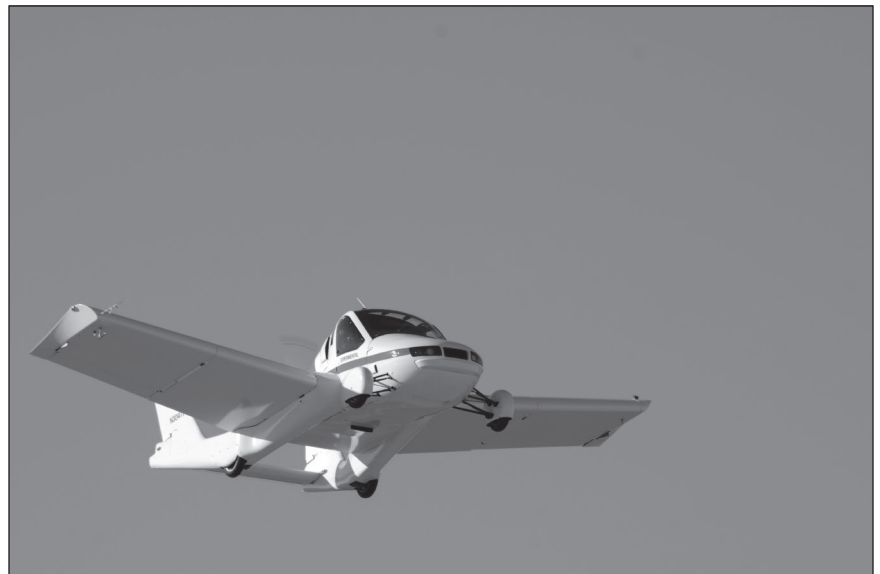
Fig. 7.30 The Transition ® car-plane in flight on March 23, 2012. It has a gross weight of 1,430 lbf and a cruise velocity of 105 mi/h. (Terrafugia, Inc.)
