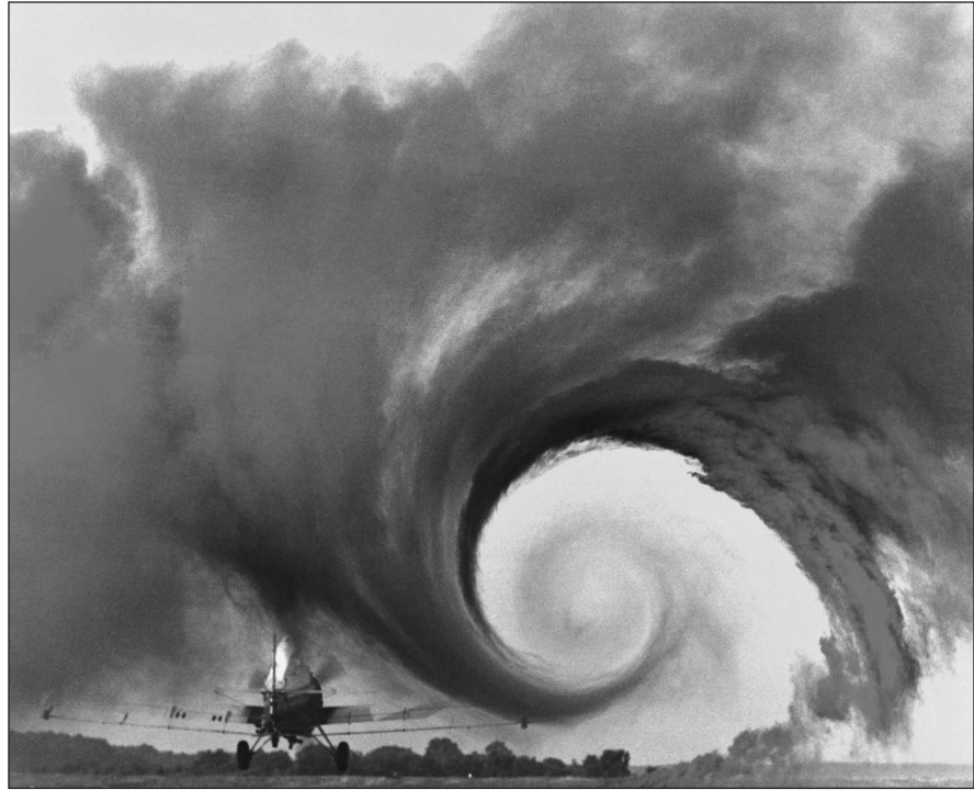
Fig. 1.19 Visualization of wingtip vortices, illustrating the huge size of the vortices produced during takeoff phase of an airplane. (NASA)
