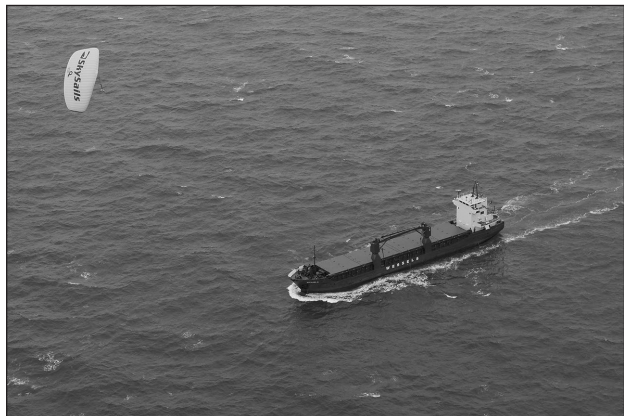
P7.85 Ship propulsion assisted by a large kite. (Courtesy of SkySails, Inc.)
