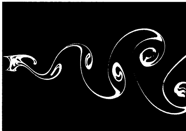
Figure 1.1. The Von Karman vortex street behind a cylinder placed in a uniform flow. (Courtesy of Sadotoshi Taneda.)
