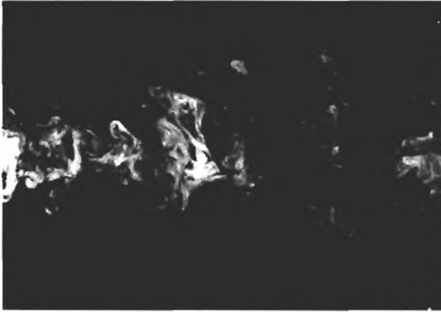
Figure 7.7. Image showing scalar concentration in a turbulent jet based on measurements using fluorescent dye. Data analysis indicates that contours of constant concentration are fractals. (Prasad and Sreenivasan (1990), reproduced with permission.)
