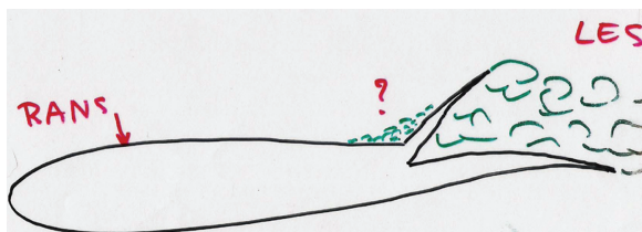
Fig. 10.13 A sketch by Philippe Spalart during early work on Detached Eddy Simulation, demonstrating the motivation for a methodology capable of operating in both RANS and LES modes, but identifying the ‘grey area’ problem in the region between the two (Spalart et al. , 1997).
