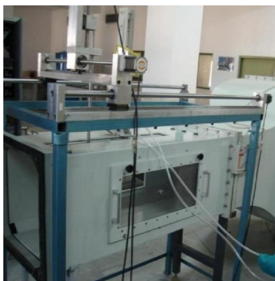
Fig. 2. wind tunnel test section and traverse mechanism.
