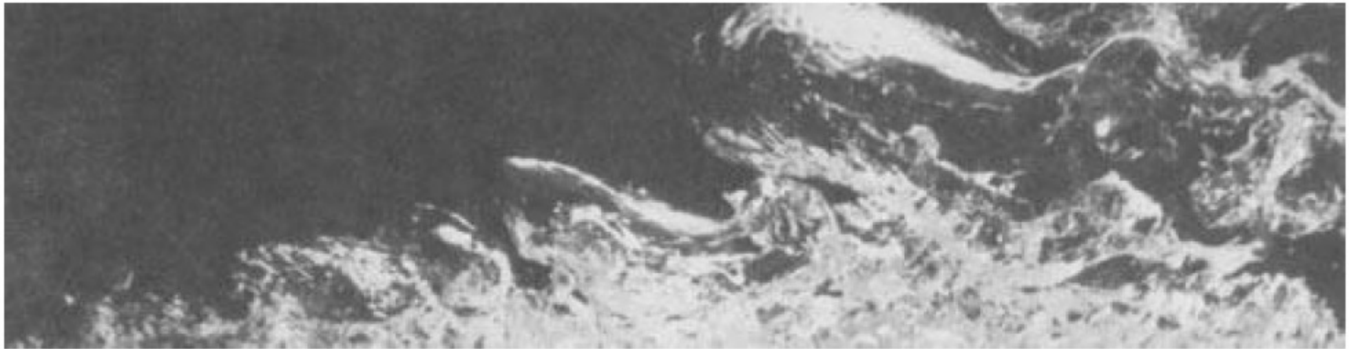
Figure 7.1 Turbulent boundary layer in boiling water flowing from left to right over a flat surface; U_\infty = 0.52 \text{ m/s} , q''_0 = 4.8 \times 10^5 \text{ W/m}^2 . (Reprinted with permission from J. H. Lienhard, A Heat Transfer Textbook , 1981, p. 417. Copyright © 1981 Prentice-Hall, Inc.)
