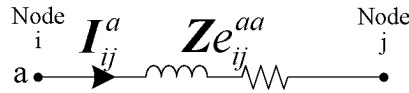
Fig. 20. A single-phase distribution feeder in a microgrid, with phasors in boldface font.
