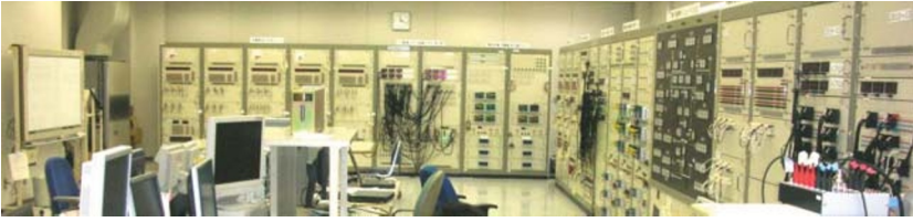
Figure 3.22 Analog power system simulator as an HIL-based power system laboratory in Kyushu Power Electric Co. (Fukuoka, Japan, June 2010).
