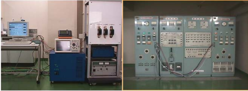
Figure 3.22 Analog power system simulator as an HIL-based power system laboratory in Kyushu Power Electric Co. (Fukuoka, Japan, June 2010).
