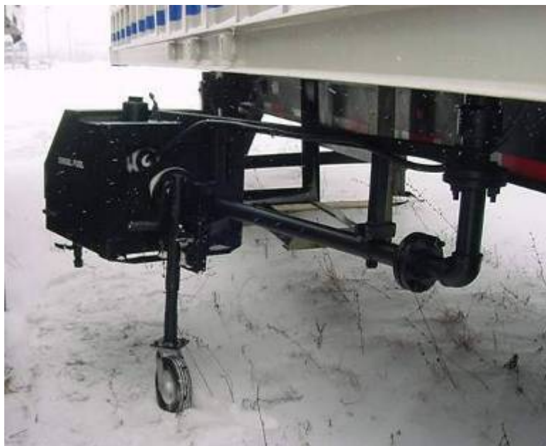
Figure 4-3 External Fuel Box: Full Pivot to Allow 6 ft. Clearance to an Opening, Break-away Pivot With Check Valve, Wheeled Support
