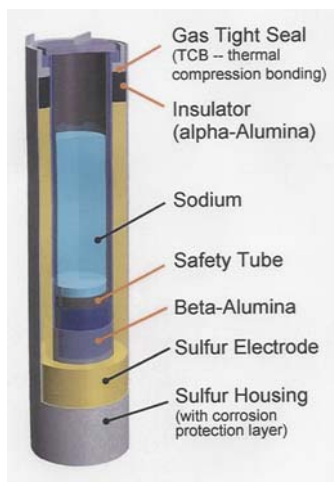
Figure 2-1 NAS Cell Components and Module
