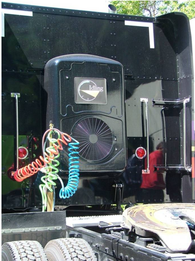
Figure 6-6 Idling Solutions System Installed on Back of Cab
