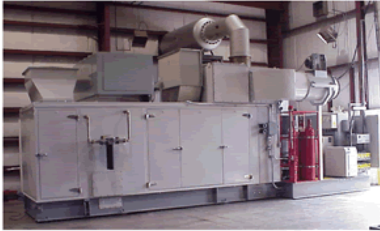
Figure 3-2 Kawasaki Combustion 1.5 MW Turbine genset equipped with Catalytica's Xonon Technology to Reduce Emissions
