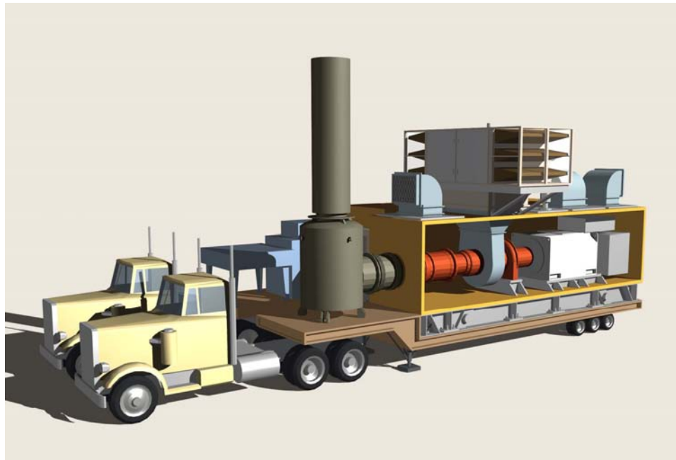
Figure 3-1 Solar Turbine's Taurus 60 Transportable Power Unit
