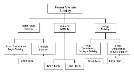
Fig. 1. Classification of power system stability.
